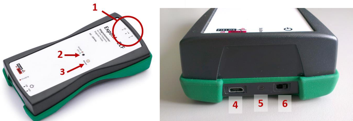
Figure 1: ExpoM – ELF elements and controls: Magnetic field sensor orientation information (1) Multi-color LED (2), Marker button (3), Micro-USB interface (4), Charging indicator LED (5), ON/OFF switch (6)
